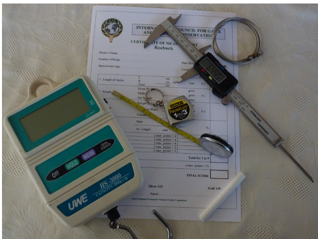
fig. 4-A: Measuring instruments for trophy evaluations. From left to right: Scales, 5 mm measuring tape and roller tape, calipers, round steel cable
